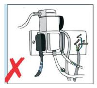
Protection Against Electric Shock - All circuits must be fully protected by Residual Current Devices with a 30 mA trip. Working on live circuits is not permitted at any time. Wooden junction boxes & Switch boards are strictly not allowed
